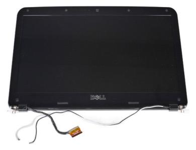
9. Using a plastic scribe, remove the six rubber screw covers from the display assembly.
