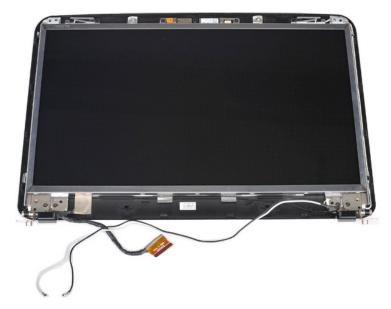
10. Remove the four screws that secure the display panel to the display assembly.
