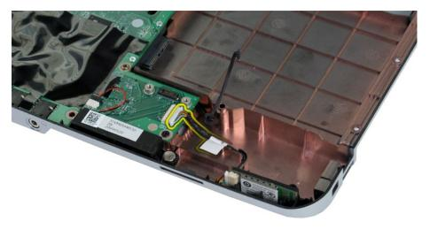
12. Release the Bluetooth card cable from its routing groove and lift the Bluetooth card to remove it from the computer.
