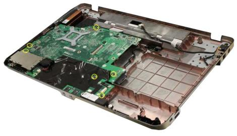
19. Lift the system board up and away from the computer chassis.
