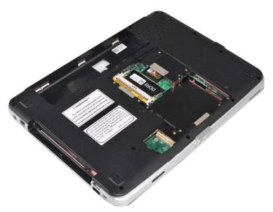
10. From the bottom of the computer, remove the screws that secure the palm rest to the computer.
