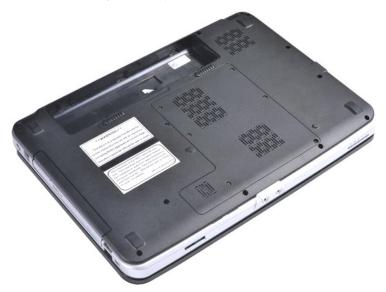
$\ensuremath{\mathsf{3}}.$  Remove the six screws that secure the access panel to the computer.
