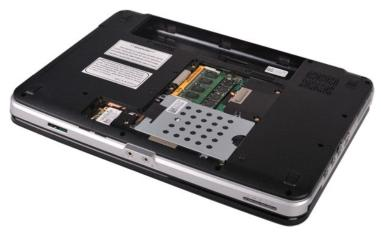
4. Remove the four screws that secure the hard drive assembly to the computer.
