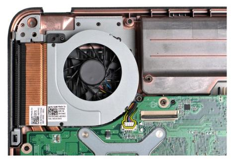
11. Remove the screw that secures the processor fan to the computer.
