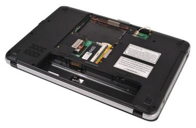
3. Remove the eight control panel cover screws from the bottom of the computer.
