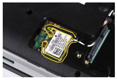
6. Remove the screw that secures the WLAN card to the computer.
