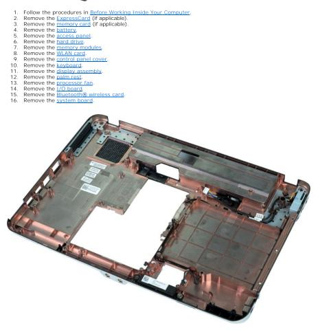
17. Remove the screw that secures the speaker to the computer chassis.
