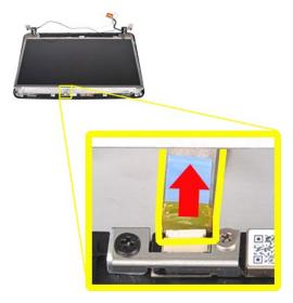
12. Lift the display LED panel from the display assembly.
