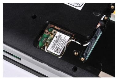
5. Disconnect the antenna cables from the WLAN card.
