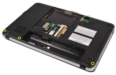
4. Insert a plastic scribe to release the four control panel cover clips located inside the battery well.
