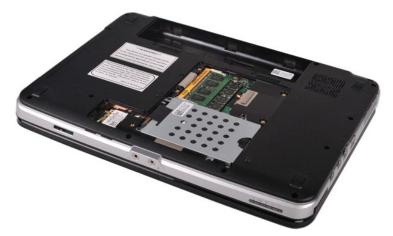
4. Use your fingertips to carefully spread apart the securing clips on each end of the first memory module connector until the first module pops up.
