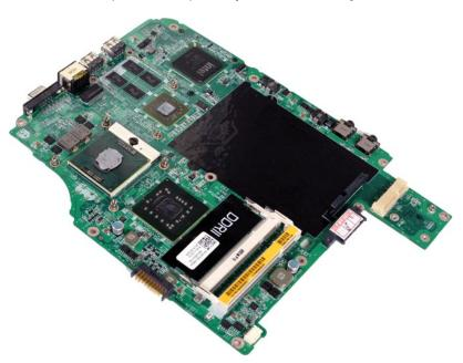
19. Use a small, flat-blade screwdriver and rotate the ZIF-socket cam screw counterclockwise until it comes to the cam stop.
