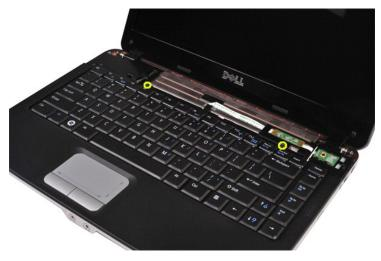
5. Flip the keyboard over and lay it on the palm rest.
