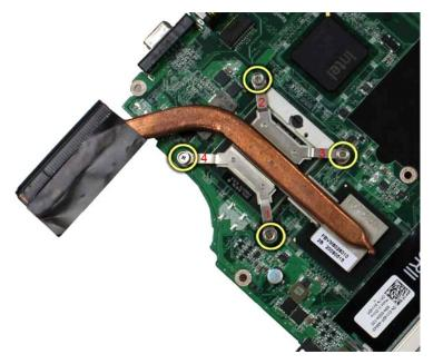
18. Remove the heat sink from the system board.
