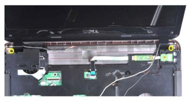
14. Lift the display assembly from the computer. Ensure that all the cables are carefully removed away from the computer.
