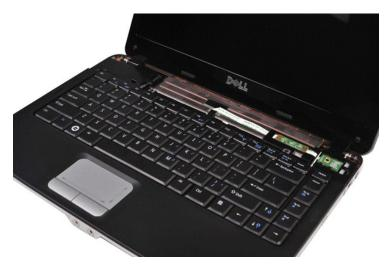
4. Remove the two screws that secure the keyboard to the computer.
