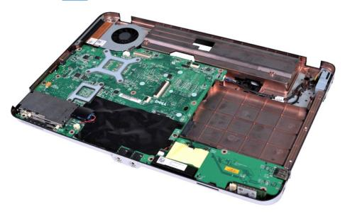
10. Disconnect the processor fan cable from the connector on the system board.
