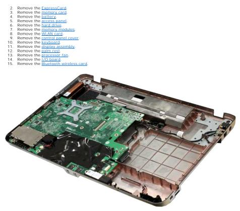
16. Disconnect the speaker cables from the system board.
