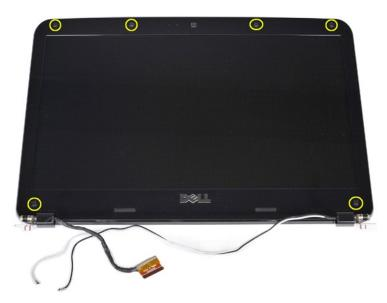
10. Remove the six screws from the display assembly.
