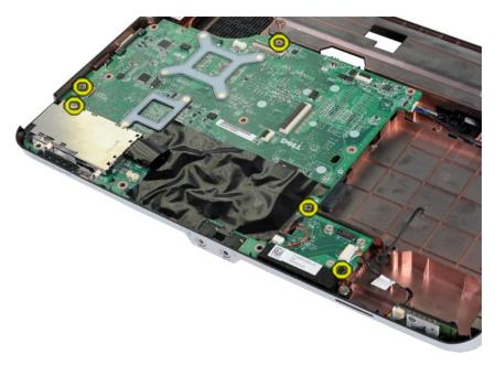
19. Lift the system board up and away from the computer chassis.
