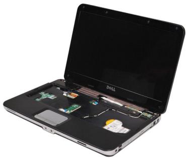
11. Remove the wireless cable from the routing guides.
