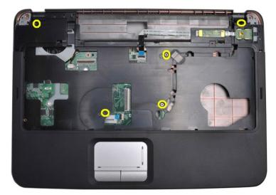
14. Disconnect the control panel and palm rest cables from the system board.
