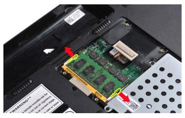
5. Slide the first memory module from its socket and remove the module from the computer.
