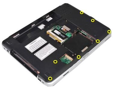
11. Remove screws that secure the palm rest to the computer in the media bay.
