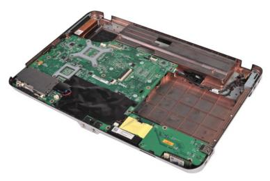
10. Remove the two screws that secure the I/O board to the computer chassis.
