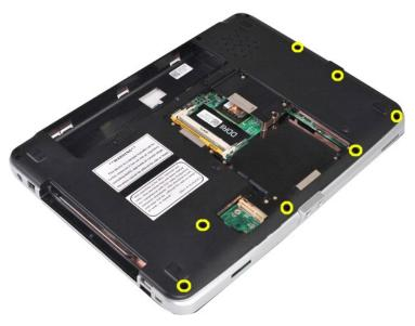
11. Remove the screws that secure the palm rest to the computer in the media bay.
