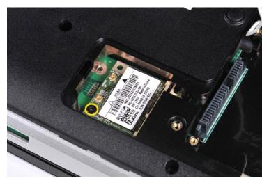
7. Slide the WLAN card out of the connector on the system board at a 45-degree angle.
