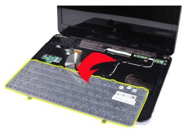
6. Rotate the keyboard data clip to release the keyboard cable from the connector on the system board.
