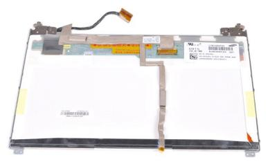
12. Carefully detach and remove the display inverter cable from the display LED panel.
