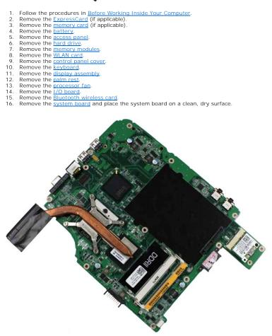
17. Use the marked sequence in the illustration below to loosen the four screws that secure the heat sink to the system board.
