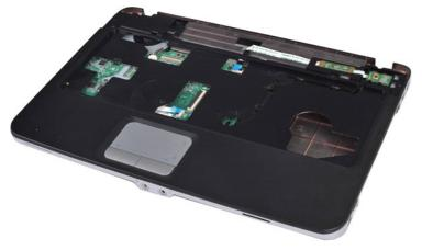
13. Remove the screws that secure the palm rest to the computer.
