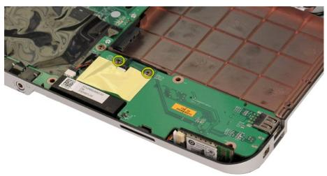
11. Disconnect the modem cable from the connector on the I/O board.
