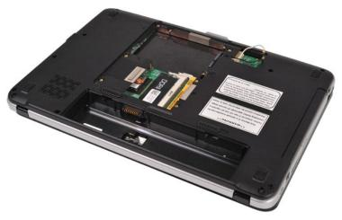
3. Remove the three control panel cover screws from the bottom of the computer.
