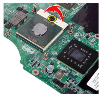
20. Remove the heat sink from the system board.
