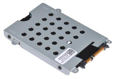
5. Remove the four screws, two on either sides of the bracket, that secure the hard drive to the hard drive bracket.
