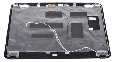
11. Remove the two screws that secure the display camera to the display assembly.
