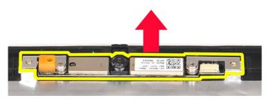
13. Remove the two screws that secure the bracket to the display camera.
