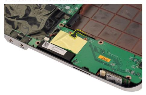
12. Lift the I/O board to remove it from the computer.
