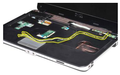
12. Rotate the display inverter cable clip to disconnect the display inverter cable.
