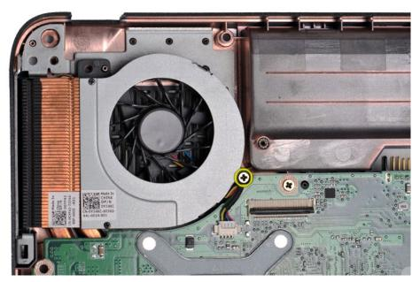
12. Lift the processor fan from the computer.
