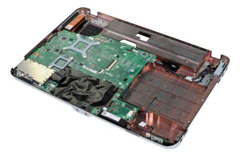
11. Disconnect the Bluetooth card cable from the connector on the system board.
