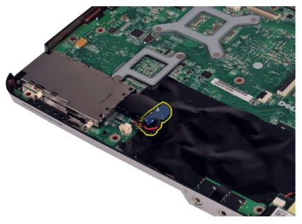
11. Disconnect the coin-cell battery cable from the connector on the system board, then lift the coin-cell battery to remove it from the computer.
